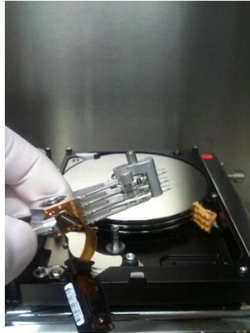
4. When the head exchange is finished, it is time to place the cover back onto the hard drive housing. When fastening the screws onto the housing, we use almost the same method as we did removing them. When tightening the screws, the first cycle is to get the screws to apply minimum pressure on the cover. The second cycle is to snug the screw (two fingers on the screwdriver tight)
